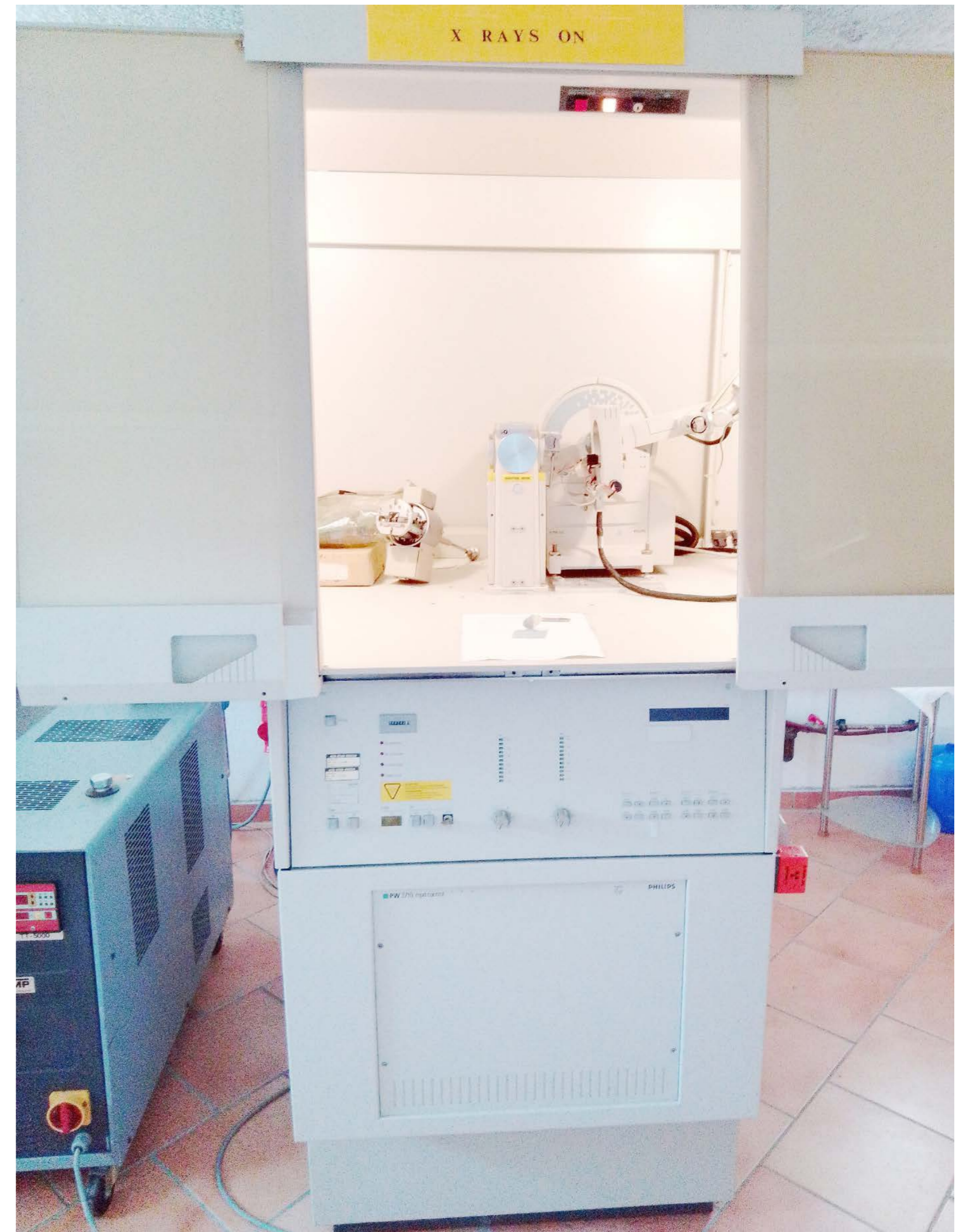
Complete XRD system. From bottom to top are the control electronics, high-voltage generator and radiation protection cabin. Through the open doors of the cabin one can see the measuring unit, consisting of X-ray tube, Euler cradle, 2 theta/theta goniometers and counting unit.
