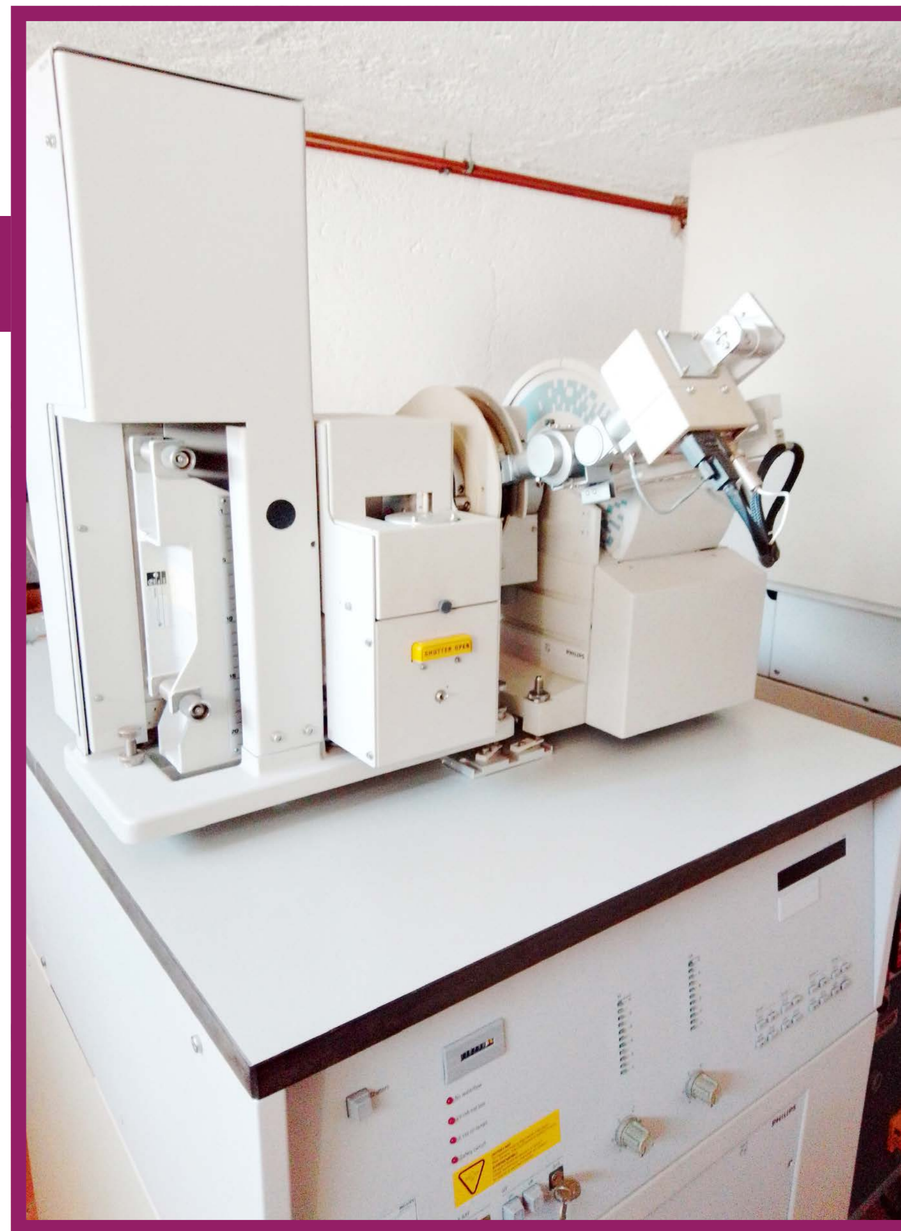
XRD device for phase analysis measurements. The measuring device with goniometer, counter, Debye-Scherrer camera, X-ray tube and sample changer is placed on top of a high voltage generator.
